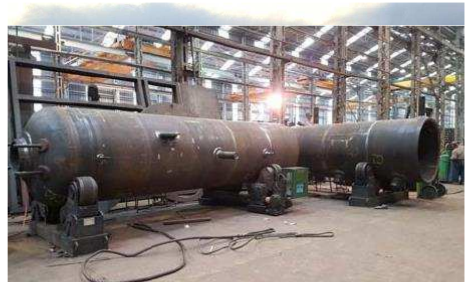
08/05/17 - HRSG (Boiler) Construction at Ricca's (supplier) site
